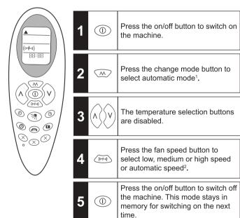
note<sup>1</sup>: In this mode the machine manages the compressor, heat pump and fan speed entirely automatically by comparing the set temperature with the internal temperature according to table A.
