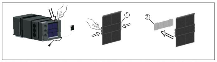
Filters cleaning (1): periodically carry out this operation; wash the filters (N.1) with a detergent solution and allow to dry before refitting. Active Carbon filter (2) (optional): It's recomended to change the active carbon filters (N.2) every year.
