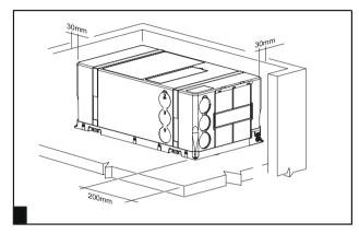
To install the machine it is necessary to create openings in the floor. The openings in the floor of the vehicle must be accessible and, therefore, must not be covered by parts of the chassis frame behind or the like.
