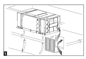
Make a hole in the compartment where the machine has been installed to permit recirculation of the internal air; Close this hole with a grille supplied that allows at least 300cm² of air to pass through. Install the condensation drain pipes provided, connect the receiver extension to the machine and lastly power up by inserting its plug into a socket outlet 220V - 50Hz.
